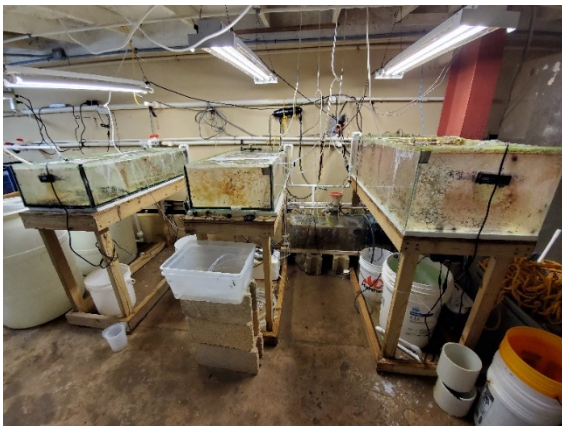
Figure 3 Seawater system containing the two 45-gallon and 60-gallon aquarium for the Diadema antillarum settlers.
