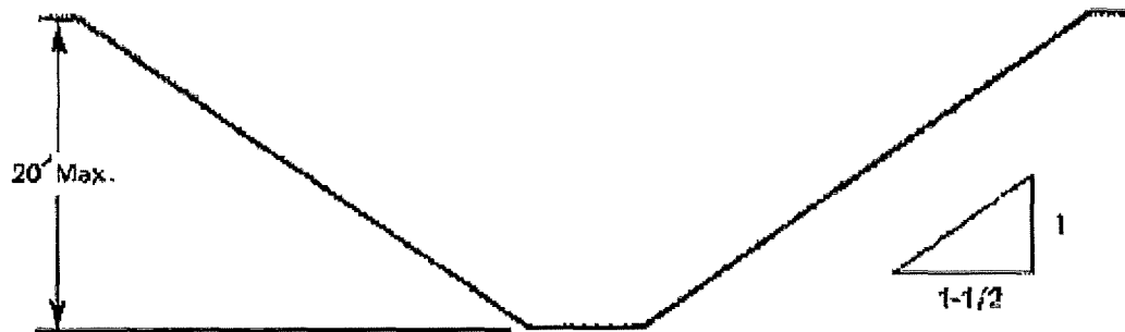
Figure 1. Excavations Made in Type C Soil
