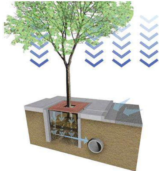
Figure 31. Diagram of a Bioretention adapted from the Houston-Galveston Area Council.
