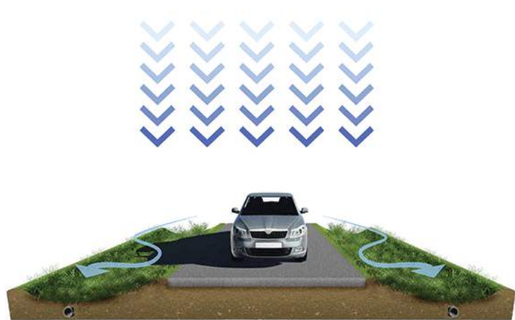
Figure 32. Diagram of a Bioswale adapted from the Houston-Galveston Area Council.
