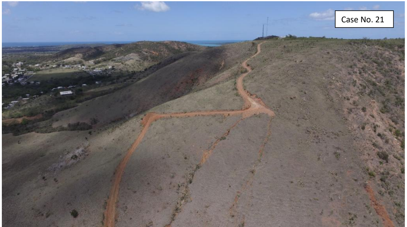
Figure 1. Erosion by unpaved road and runoff water.
