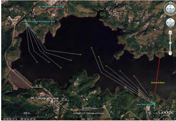
FIGURE 1. Final design of ORS installed in Toa Vaca Reservoir. Note that 10 diffusers were installed, not the original 14 proposed. Image credit unknown; provided by: Craig Lilyestrom and Miguel A. Garcia Bermudez, DNER.
