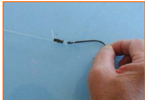
Figure 3.3-22f. Tag end may be trimmed to form "pin"
