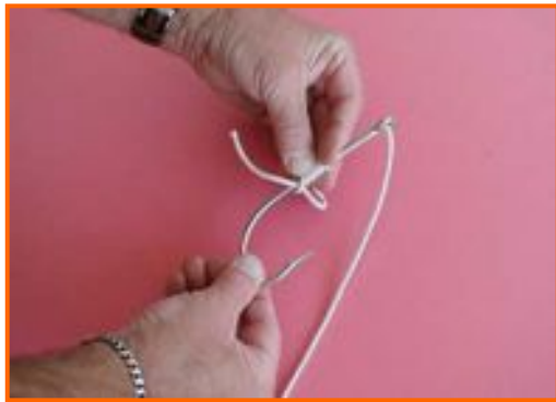
Figure 3.3-31c. Insert tag through loop at bend of hook
