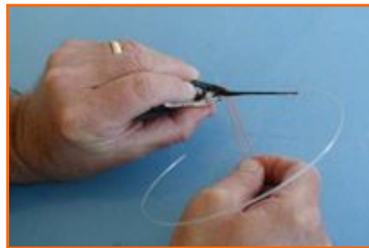
Figure 3.3-26f. Loop rubber band over pin and wrap it twice around the head
