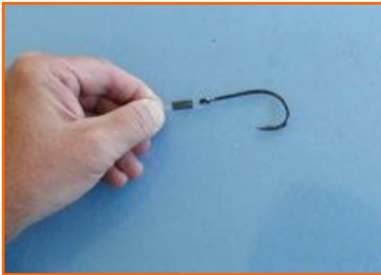
Figure 3.3-22c. Push crimping sleeve close to hook
