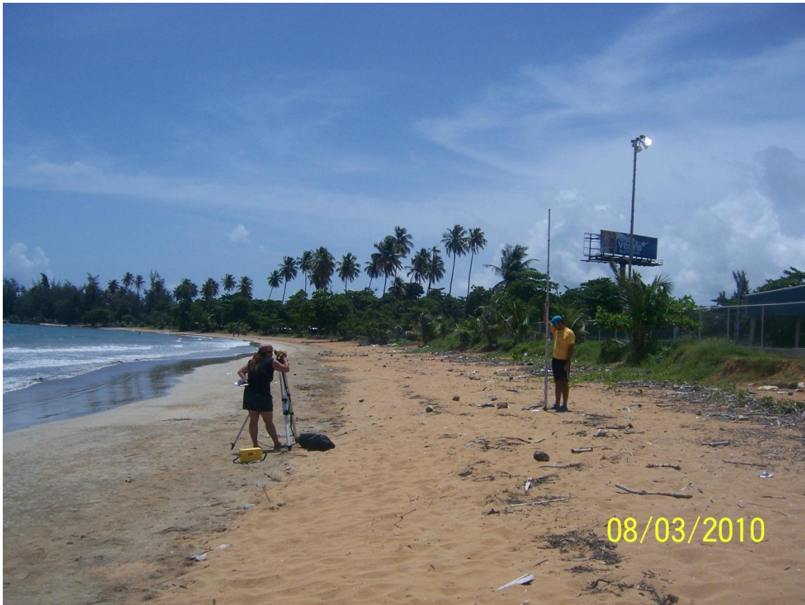
Figure 45. Beach profile 1 at Playa Fortuna. Dissipative profile was observed near to recreational infrastructure in the study site during August 2010.
