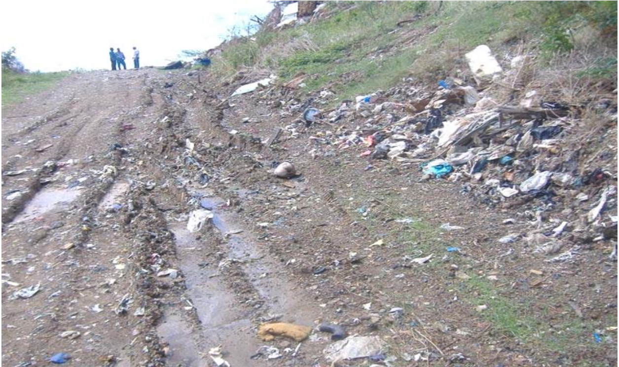
Photographs No. 13 & 14- Looking to the west showing two leachate-prone surface areas running to the southeast. This area is identified as leachate Zone Z-1
